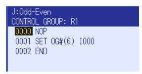
Now that the variable is written to the output group, all we need to do is monitor the first bit of that group, in our case Output#41. If it is on, the value of the variable must be an odd number. If it is off, the value must be an even number. We can monitor this with an if then statement and continue our programming.
